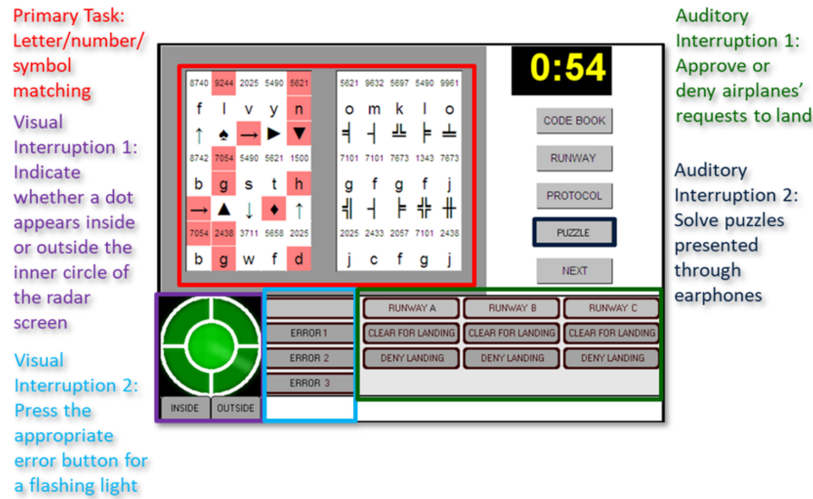
Figure 15 Labeled Snapshot of the Control Tower Interface
